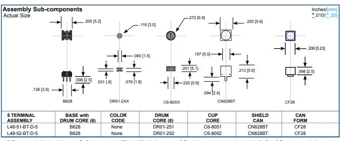
6) "The base is molded in a phenolic thermoset. The 5 terminals are brass, ".027 inches (0.7mm) in diameter, 100 % tin plated to meet MIL-STD 202 method 208 for solderability."
